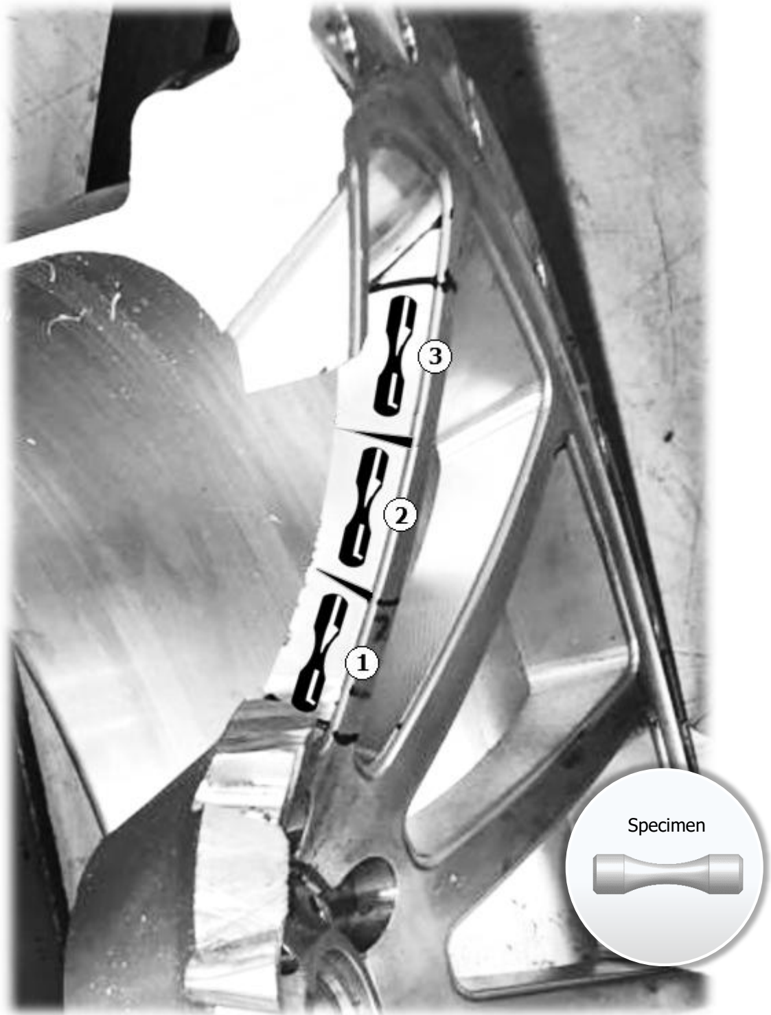
Figure 9. Cutting Samples from Wheel Rim
